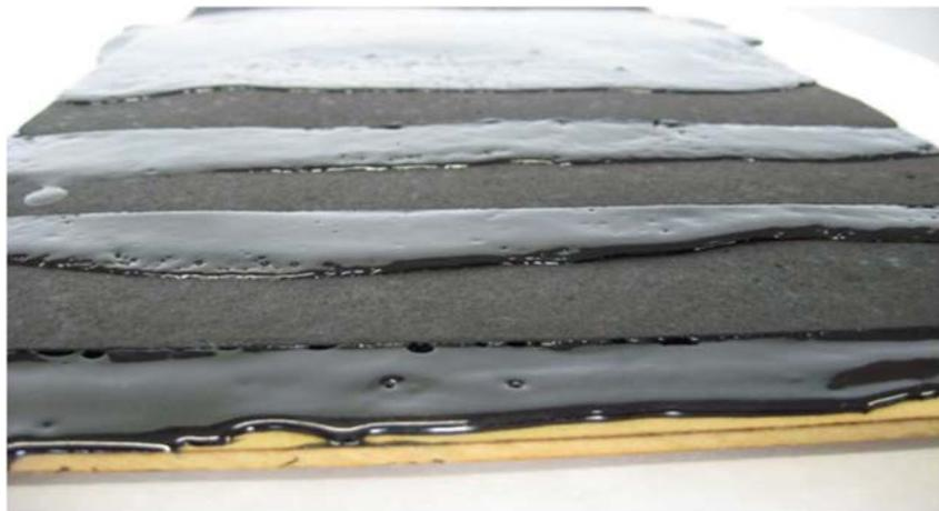
**(VECCHIO SISTEMA) 3 STRATI DI CARTA BITUMATA INCOLLATI CON 4 SPALMATURE DI BITUME FUSO**
